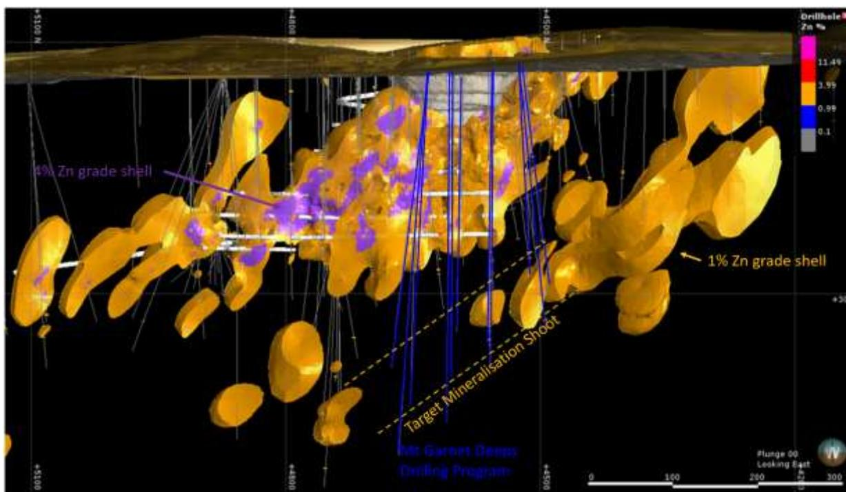
**Figure 2:** Mt Garnet Deeps drill hole plan. Image looking east. Planned drill holes in blue
