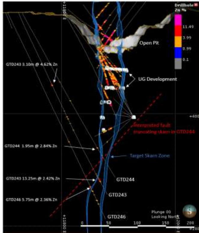
**Figure 3:** X-Section A showing recent drilling results. Image looking north
