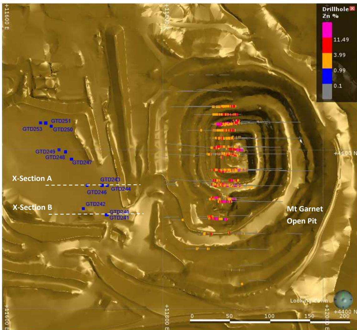
**Figure 2:** Mt Garnet Deeps drill hole location plan. Planned drill holes in blue
